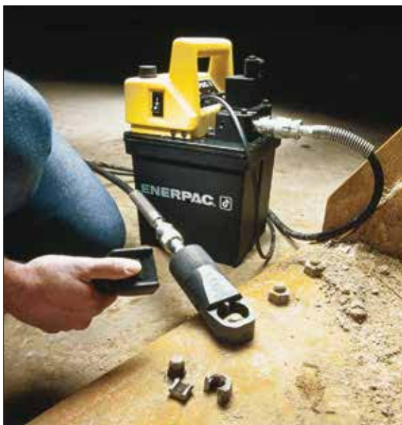
◀ This PED-1101E Submerged pump quickly and quietly powers a hydraulic nut cutter in this bucket maintenance application.
