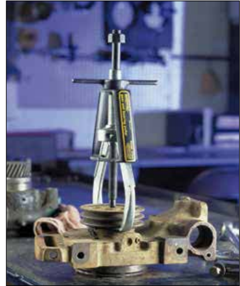
▲ EP-204 2 jaw puller positioned to pull a water pump drive pulley.
