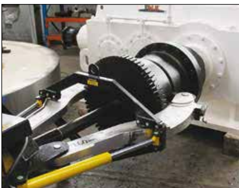
◀ The EPH-1002E quickly and easily removes this drive coupler from its shaft.
