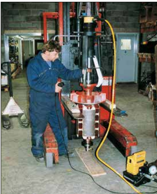
◀ EPHR-116 used to remove electric motor pulleys. Puller is positioned using the Lift Plate.
