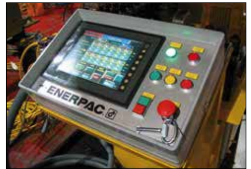
▲ PLC-controller station for ESS-Series synchronous lifting system.
